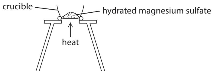
**Step 3** After heating for two minutes, the crucible containing the magnesium sulfate was allowed to cool and was reweighed.
